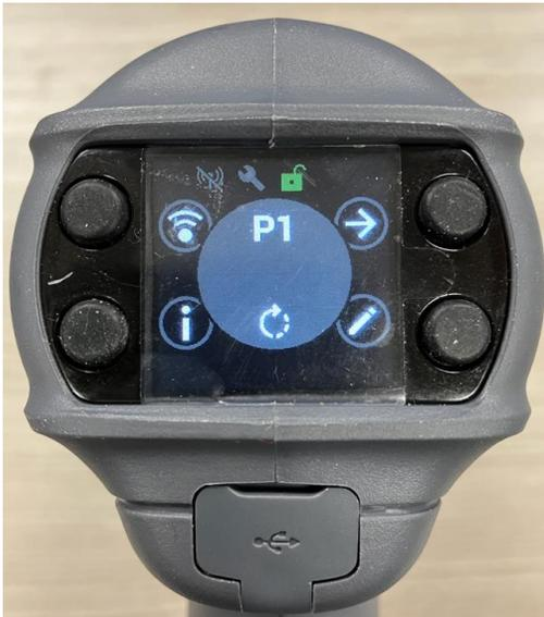
9. Press the button next to the right arrow icon to select the desired Pset. The following screen shows Pset 3 with Batch Count = 4 and CCW Direction.
