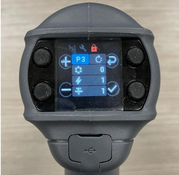
4. Press the button next to the Navigation icon to move to the next field. You will see the following screen with the Direction field highlighted. The Direction was changed to CCW using the buttons next to the + or – icons.
