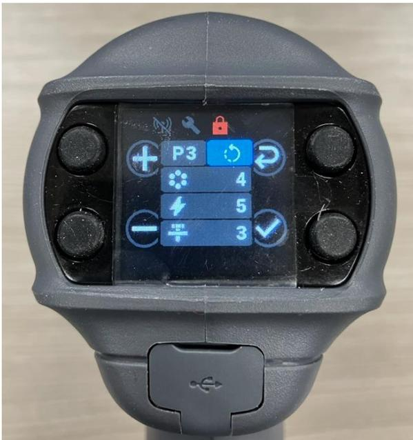
5. Press the button next to the Navigation icon to move to the next field. You will see the following screen with the Batch Count Field highlighted. The Batch Count was set to 4 using buttons next to the + or - icons.
