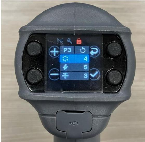
6. Press the button next to the Navigation icon to move to the next field. You will see the following screen with the Torque Level Field highlighted. The Torque Level was set to 5 using buttons next to the + or - icons.
