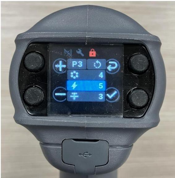
**Torque Level Setting (T1 – T40)** – This setting is the duration after flush point detection during which the tool delivers pulses of torque to the fastener before automatically shutting off. There are 40 options to choose from, so that the tool's delivered torque may be best aligned with the torque that the application requires.
