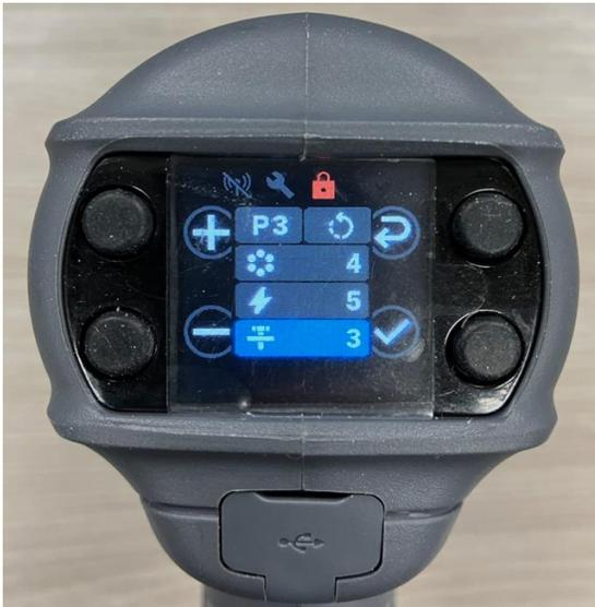
**Flush Level Setting (L1 – L7)** – This setting is the level of sensitivity used for determining when the flush point has been reached. Since all joints are different, there are 7 options available to choose from, so that the tool’s determination of flush point may be best aligned with the actual joint behavior.
