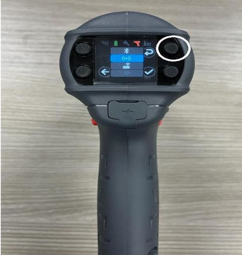
7. Press the button next to the Check Mark to put the tool into Pairing Mode.
