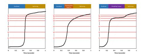
d. Torque Level Setting (T1 – T40) – This setting is the duration after flush point detection during which the tool delivers pulses of torque to the fastener before automatically shutting off. There are 40 options to choose from, so that the tool's delivered torque may be best aligned with the torque that the application requires.
