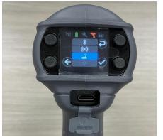
18. Press the button next to the Check Mark to put the tool into Pairing Mode.
