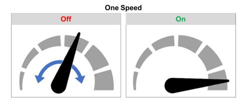
j. **Soft-Start** – Tool speed ramps up more gradually at the beginning of a cycle. <u>Why it is useful</u>: The gradual speed increase of soft start can provide the operator with more control for getting fasteners started.
