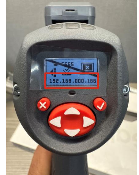
Tool Connected to Access Point Successfully
