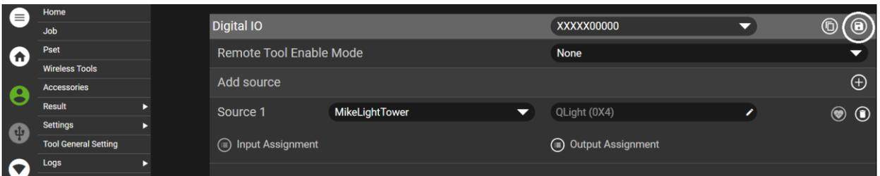
13. The Light Tower is programmed and the LEDs will illuminate after each cycle based on the programmed Behaviors, Timer and Blink status.
