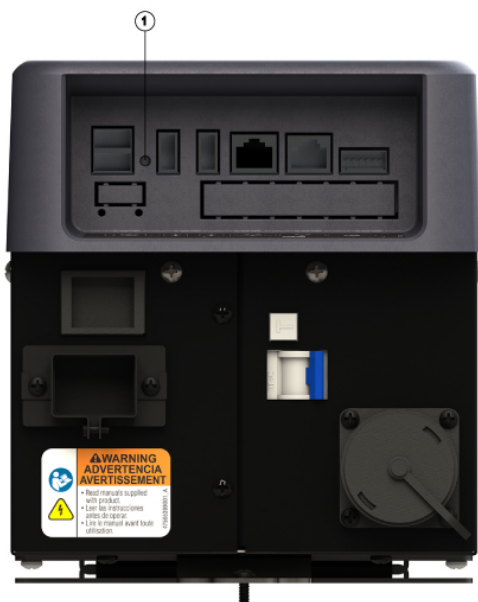
Figure A: View of IP Address Reset Pin on fastening controller
