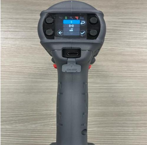
3. Press the button next to the Check Mark to put the tool into Pairing Mode.
