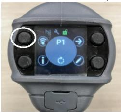
6. Press the button next to the return icon to navigate to the Radio icon from the tool backcap.
