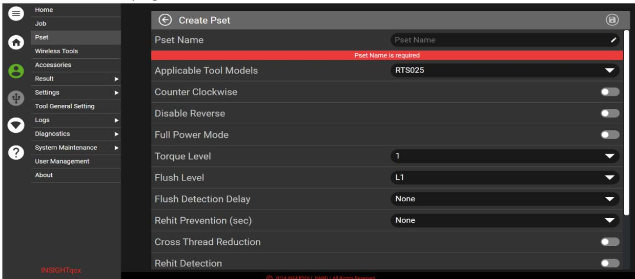
3. At a minimum, Pset Name, Tool Model, Torque Level and Flush Level should be programmed.
