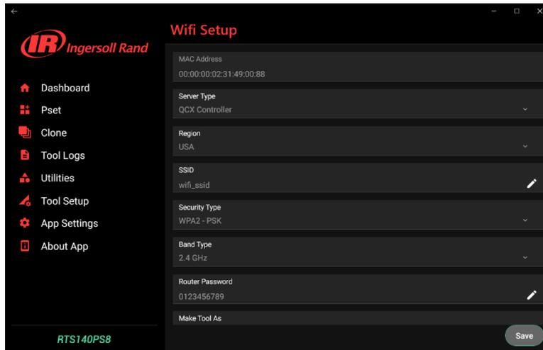
h. Enter the router WiFi settings (SSID, Password, Security Type, and IP Mode).
