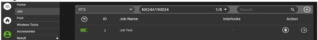
13. Go to the Home screen and the Job will be available in the Drop Box. This is the case as long as the Job Selection Mode is Internal Controller on the Tool Settings screen.
