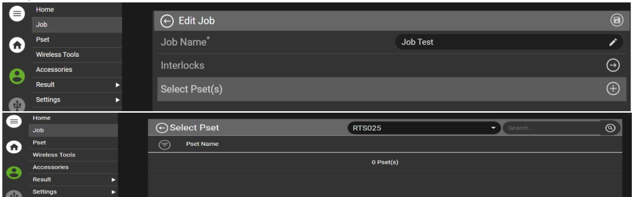
7. Select the desired tool model and assign the Pset.
