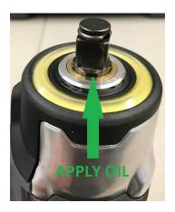
If the noise persists then remove hammer case and clean & lubricate as instructed in the Product Information manual (shown below). Apply IR 105 grease to the anvil and impact mechanism assembly. Apply IR 67 Grease to the gears.
