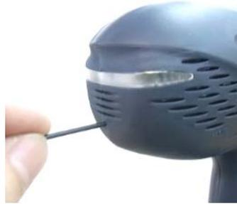
**\*Do not continue to press the pairing button after the buzzer beep and fast blinking of the LED.**
