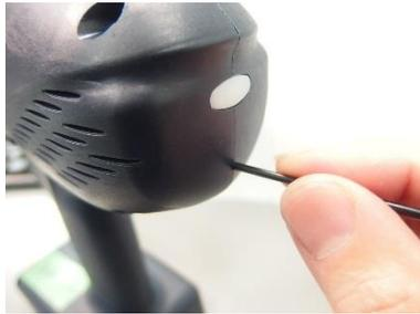
**\*Do not continue to press the pairing button after the buzzer beep and fast blinking of the LED.**
