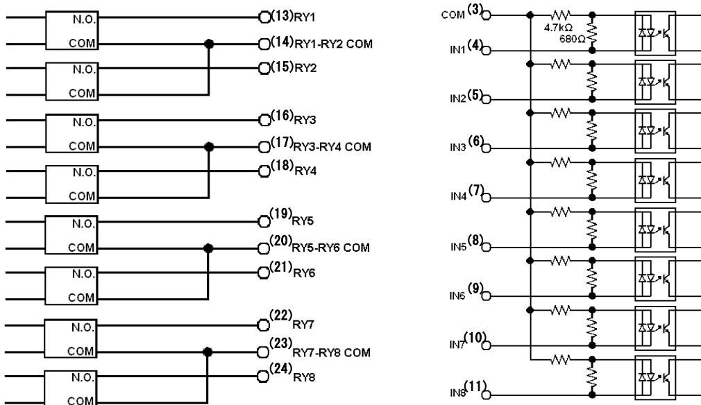
\* Current capacity available from DC 24V (Pin 1 and 2, 12) is max. 100mA in total.
