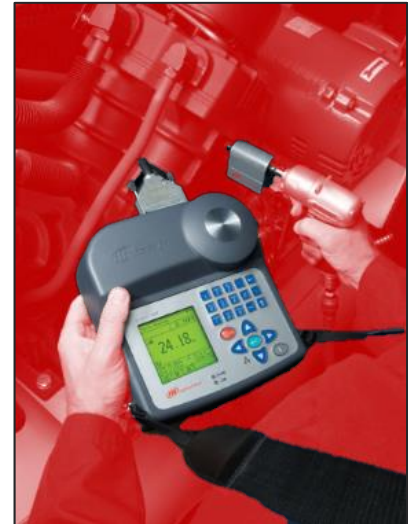
Above shows a typical validation procedure setup using an Ingersoll Rand EXTA torque analyzer and a rotary inline transducer
