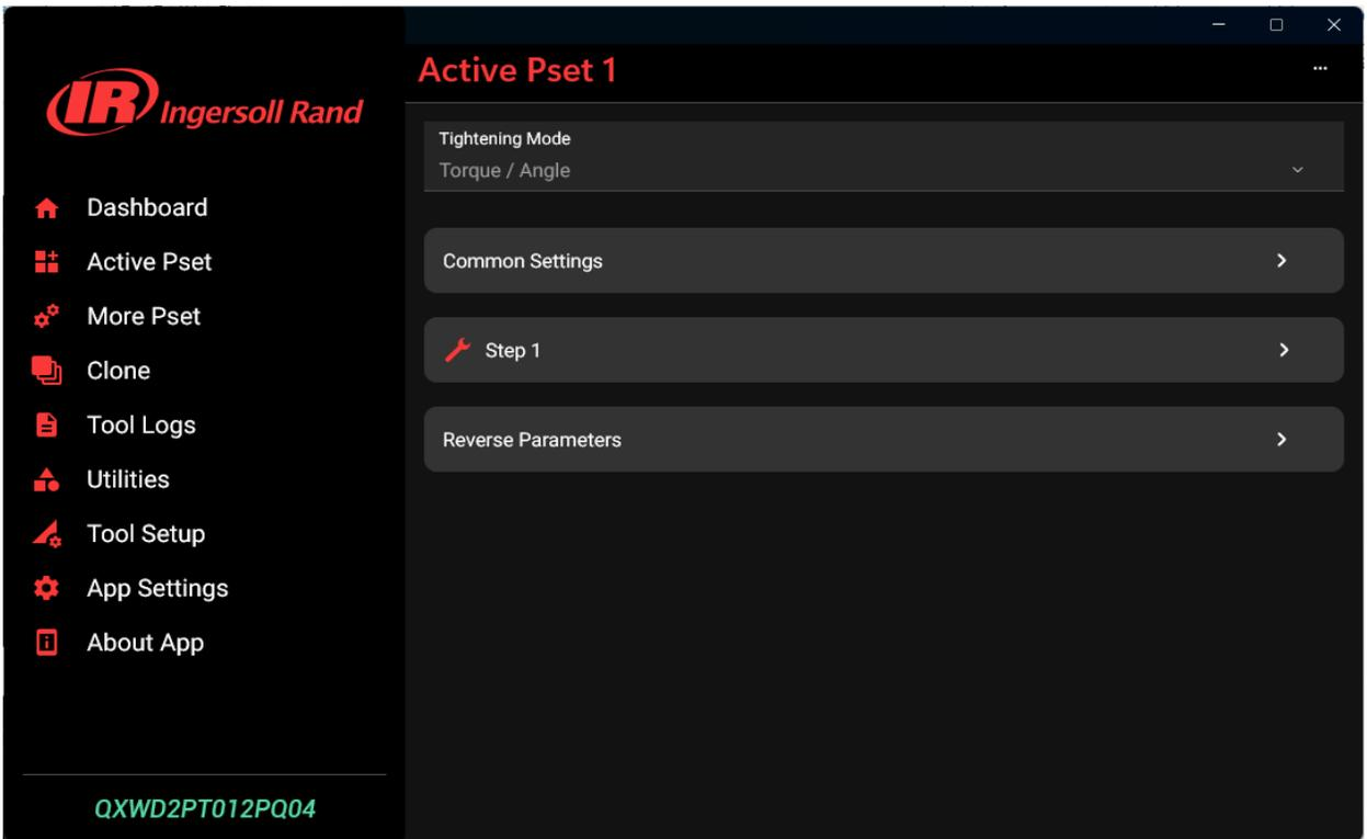
9. Click on Step 1 to view/edit the Tightening Parameters.
