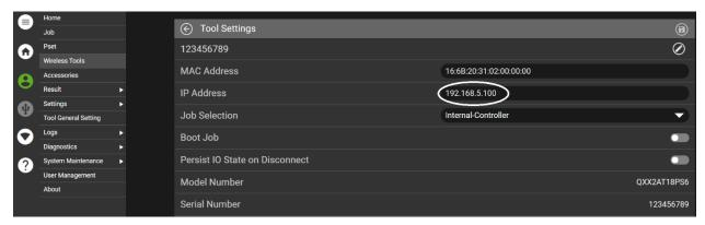
10. Sample results using IP Aliasing. Note: Unique IP Addresses assigned to each tool
