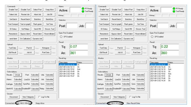
11. Sample results with IP Aliasing disabled. Note: Unique port numbers assigned to each tool
