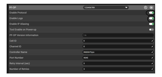
4. With IP Aliasing enabled, the controller will communicate with the Unique Tool IP Address and user given PF-OP Port number
