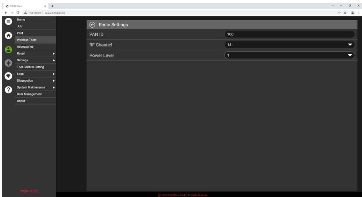
Change the RF Channel to the desired channel. In this case it will be 17. Change the Power Level to 4 for maximum power/distance. Press the arrow next to the Radio Settings heading. A popup will appear warning that the tools will be unpaired. Press the Yes button to unpair the tool(s).
