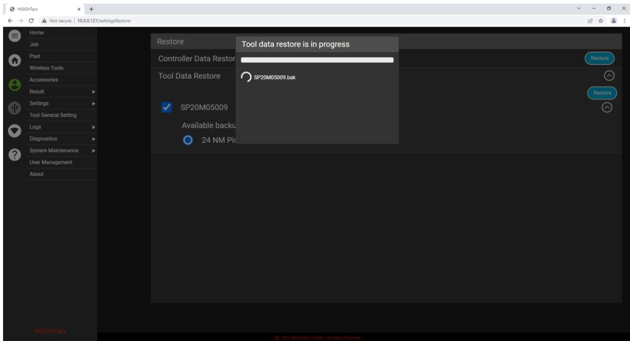
The controller will reboot when the tool backup is complete. Repeat this process for all paired tools.
