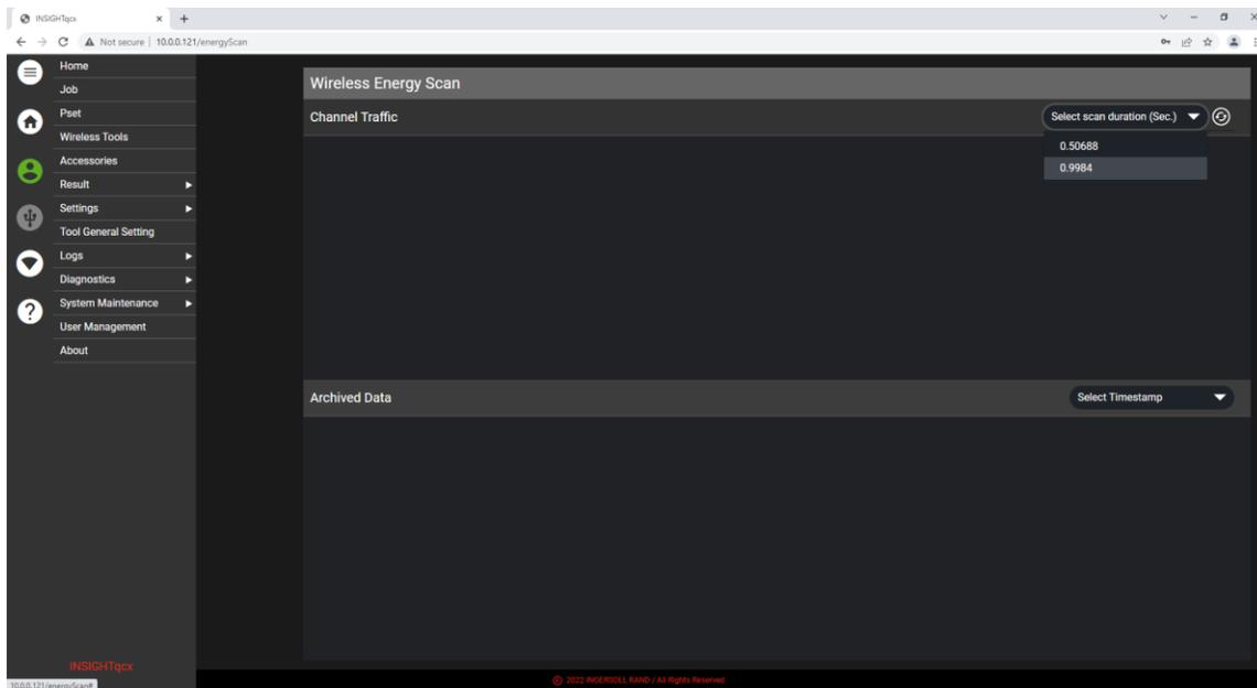
The energy scan disables communications with the tool for the duration of the scan. It is not recommended to perform the energy scan while production is running. Press the Yes button to initiate the scan.
