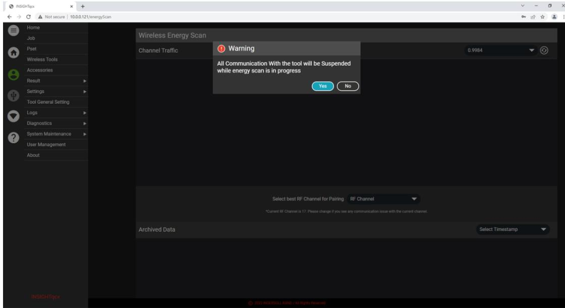
After the scan completes, a table will show with the energy levels observed on all channels. Channel 25 is used for pairing and cannot be selected. Usually channels 15 and 20 are the quietest. On the screenshot below, these channels are high as there are controllers and tools using these channels nearby. Channel 17 will be chosen for this example.
