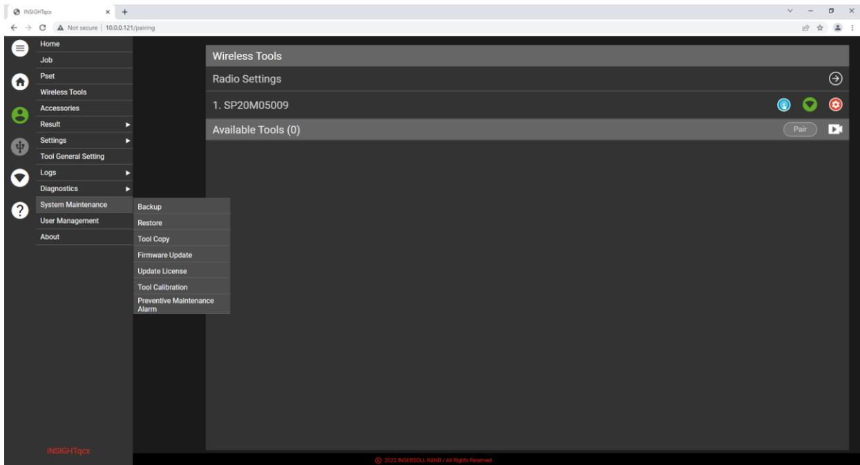
Expand the Tool Data Restore. A list of paired tools will be display. Check the box for the first tool to restore. A selection will appear with the saved tool backup files. Select the appropriate file and then press the Restore button in the Tool Data Restore pane.
