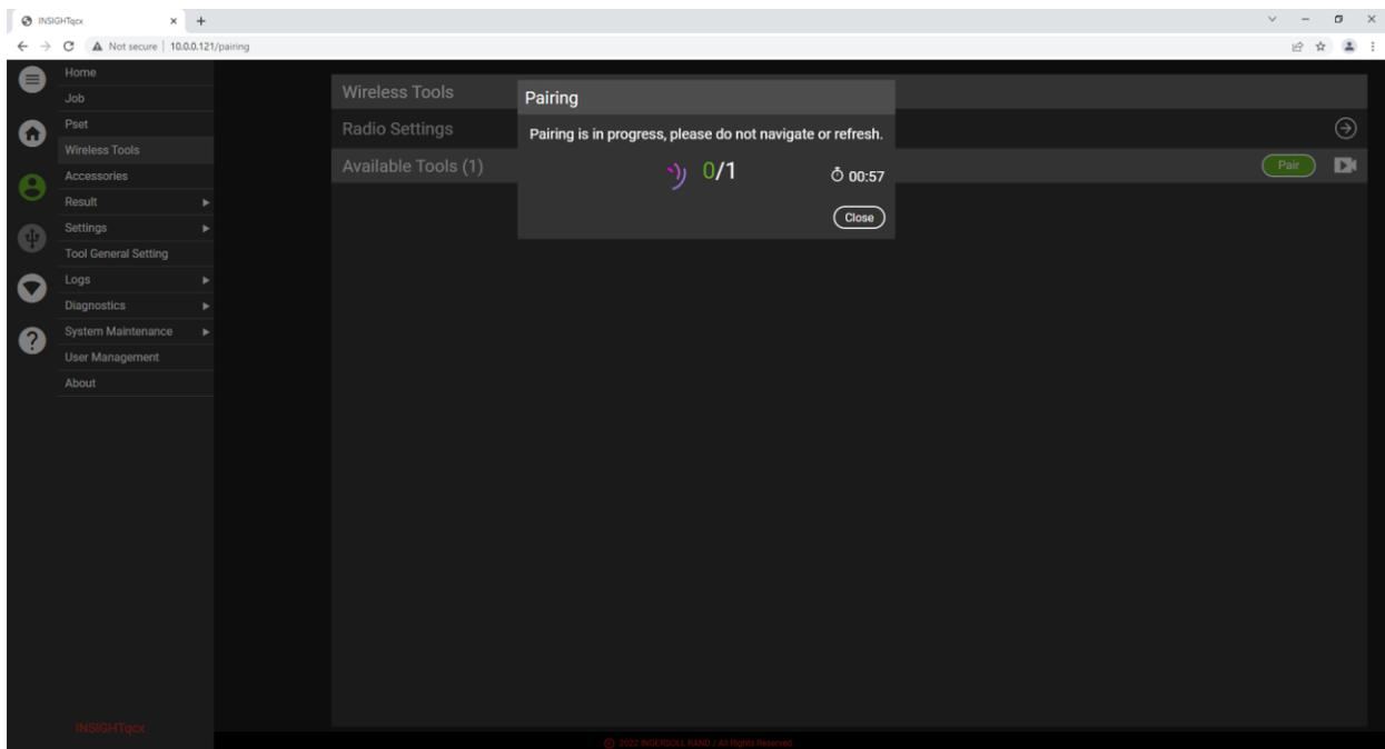
When the number of tools that you are pairing matches on the screen you can press the Close button. (For example, on a 4:1 controller and you are pairing 2 tool, as soon as the screen shows 2/4 you can
